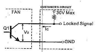
\*Transistor Q1 at "ON" position
