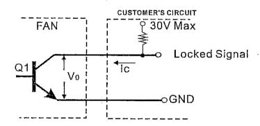
\*Transistor Q1 at "ON" position Collector current......... $I_c$ =10mA Max Saturation Voltage...... $V_{oL}$ =1.0V Max (Between Collector and Emitter at  $I_c$ =10mA) \*Transistor Q1 at "OFF" position Release Voltage...... $V_{oH}$ =30V Max
