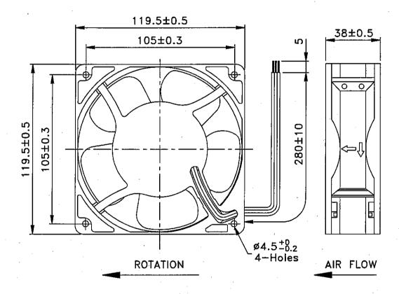
LEAD WIRES: UL 1007, AWG24, L = 280 +/- 10 MM Red = positive; Black = negative.
