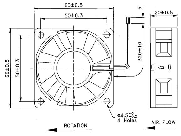
please do not touch and push Fan Blade with fingers or others. Fan Blade and Ball Bearings may be damaged. And it causes noise defect.
