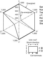
Sample: G6DN-1A Number of Relays: 5 pcs Test conditions: Impose a shock in the  $\pm X$ ,  $\pm Y$ , and  $\pm Z$  directions three times each with the Relay energized to check the shock values that cause the Relay to malfunction. Standard:100 m/s<sup>2</sup>
