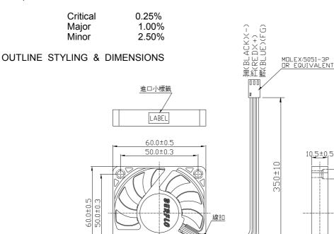
LEAD WIRES: UL 1007, AWG26, L = 350 +/- 10 mm Red = positive; Black = negative. Blue = FG
