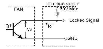
\*Transistor Q1 at "ON" position
