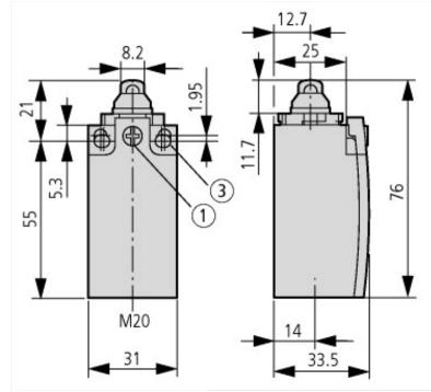
① Tightening torque of cover screws: 0.8 Nm ±0.2 Nm ② only with LS (insulated version) ③ Fixing screws 2 x M4 ≧ 30 M<sub>A</sub> = 1.5 Nm
