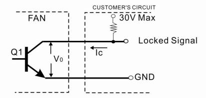
\*Transistor Q1 at "ON" position Collector current....... $I_c$ =10mA Max Saturation Voltage...... $V_{oL}$ =1.0V Max (Between Collector and Emitter at  $I_c$ =10mA)
