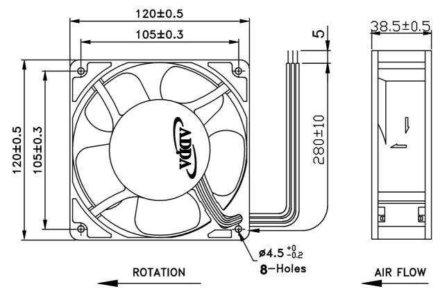
LEAD WIRES : UL 1007, AWG24 , L =  $280\pm10$  mm Red = positive ; Black = negative.
