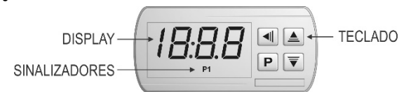
Fig. 05 – Painel frontal do controlador
