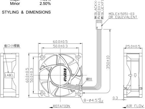
LEAD WIRES: UL 1007, AWG24, L = 350 +/- 10 mm Red = positive; Black = negative. Blue = FG
